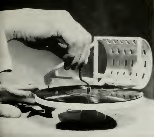
The seven-ounce, unbreakable phonograph, made largely of plastic, is operated by turning the crank.
